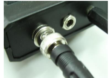
BNC Input for Accelerometer
